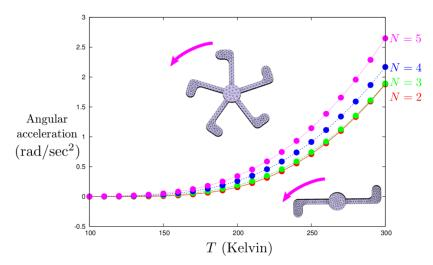
Figure 2: Angular acceleration due to self-rotation torque vs. temperature on QED pinwheels - (chiral gold nanoparticles of thickness ~ 250 nm and diameter ~ 2  $\mu$ m) embedded in a cold (0 K) environment.
